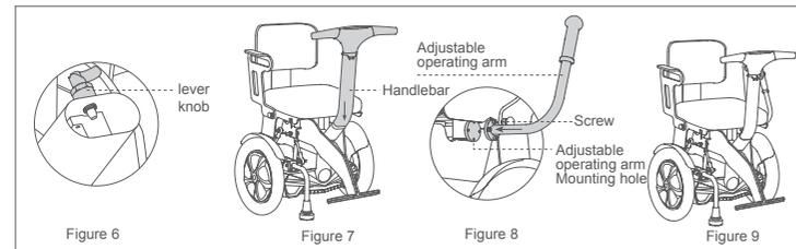
2. Rotate the lever knob, after hearing a "click", insert the handlebar (see Figure 7). Then keep rotating the lever knob until you hear a "clatter", the handlebar is installed. Take out the lift lever out of the foam box and align it with the mounting hole (see Figure 8). Tighten the screws and the body is installed (see Figure 9).
