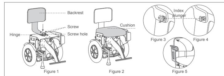
1. Take A6T from the packing container. Align the screws on backrest hinge to the screw holes and body holes, tighten screws (see Figure 1) and stick saddle to frame (see Figure 2). Pull outward and rotate the index plunger (see Figure 3) and get the mount stuck and loosen the index plunger (see Figure 4); rotate the armrests to horizontal position (see Figure 5 - arrow). Pull outward and rotate the index plunger and release it when a click sound is heard.
